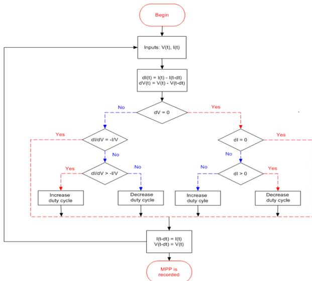
Figure 2: Incremental Conductance flowchart based MPPT
