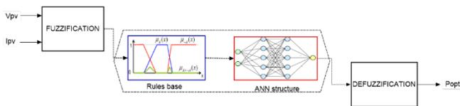
Figure 5. Architecture of the MPPT ANFIS technique
