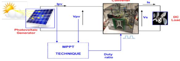
Figure 1: Schematic diagram of the MPPT technique
