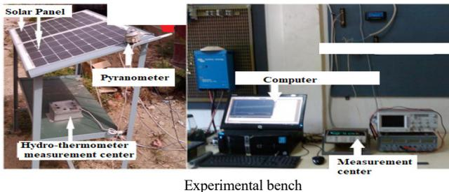
Figure 8: Experimental database of irradiation and temperature
