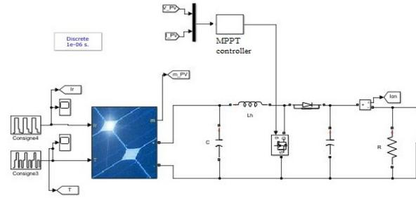
Figure 9: System simulated under matlab/simulink
