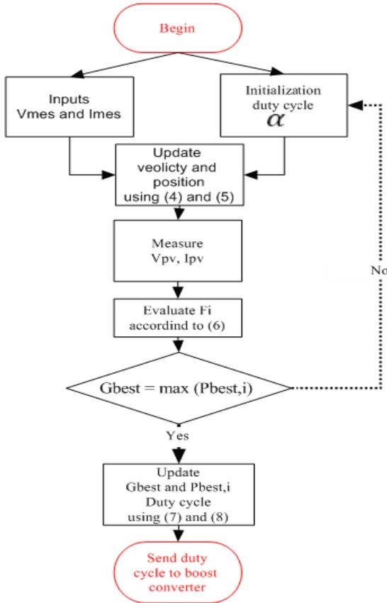
Figure 4: PSO flowchart based MPPT
