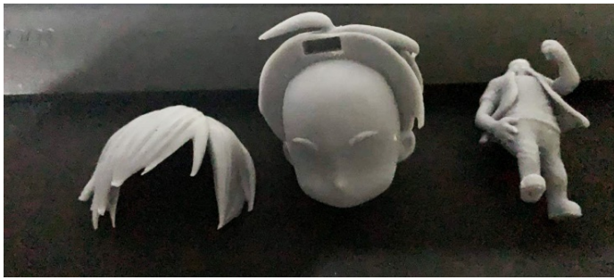
Figure 31: The test 3D model printing using resin separated 3 pieces.
