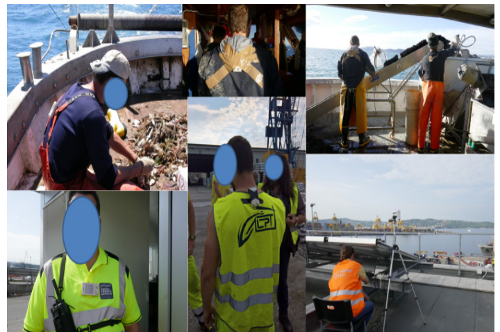
Figure 1: Placement of the UV electronic dosimeters at the workplace, on the fishermen (FM) and dockworkers (DW). From left to right, top to bottom: (1) a FM with a dosimeter on the back and one on the cap to simulate nape exposure; (2) a FM with a back dosimeter working in a covered area of the boat; (3) two FM with back dosimeters working in an uncovered area of the boat; (4) a DW working as port coordinator with a chest dosimeter; (5) a DW working as longshoreman with a
