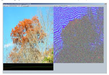
Figure 6. Image Analysis window, cover image on left, LSB analysis on the right
