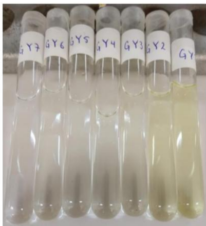
Figure 4. Color standards used for solution color testing. GY = color scale according to pharmacopoeia within the brown-yellow-red interval. GY1 represents the highest intensity.
