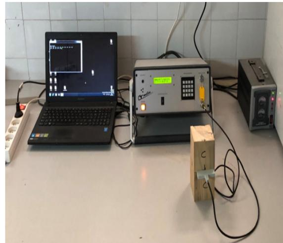
Figure 2: Launch of Araucaria samples in CT-Metre device
