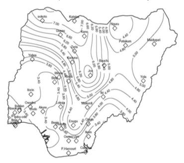
Figure 5: Nigerian wind map in m/s determined from 40 years measurements at 10m height, obtained from Nigerian metrological department, oshodi,lagos state, Nigeria(NIMET).
