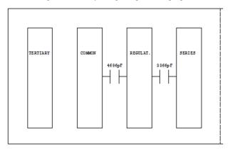
Figure 7: Autotransformer winding arrangement wye connection
