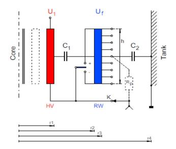
Figure 6: Recovery voltage - capacitances per phase
