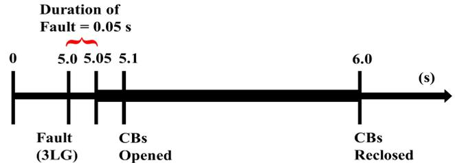
Figure 10: 3LG fault conditions.
