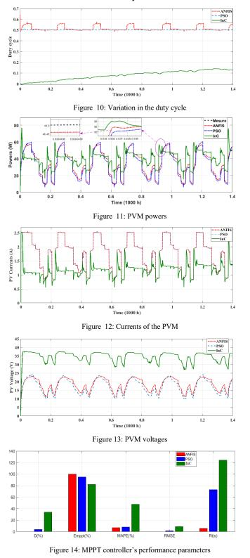
These results corroborate those found in the literature which highlight the oscillating nature of the power obtained with the InC technique due to their inability to detect with precision the overall maximum in a situation of non-uniform climatic conditions [3]. They also confirm the results presented in [38] where the authors made a comparison between ANFIS and InC.
