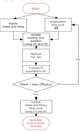
Figure 4: PSO flowchart based MPPT
