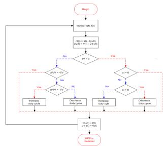
Figure 2: Incremental Conductance flowchart based MPPT
