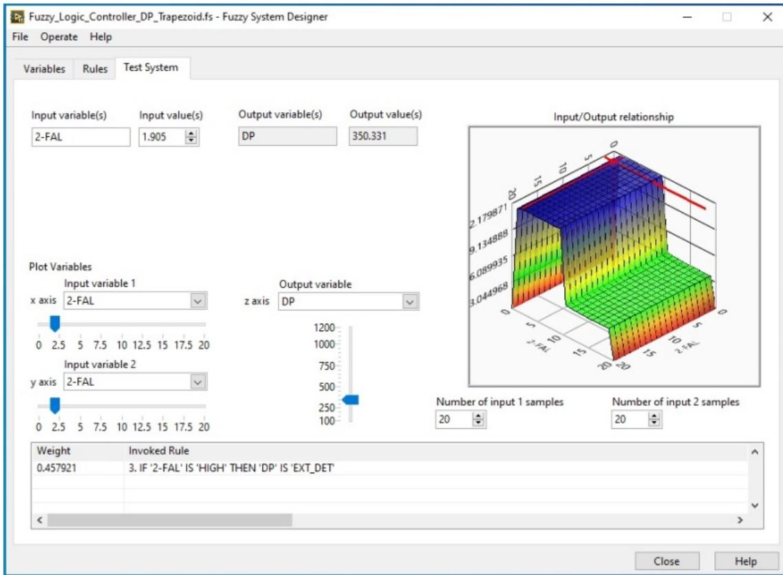
Figure 7: Surface viewer of DP result based on trapezoidal fuzzy logic controller
