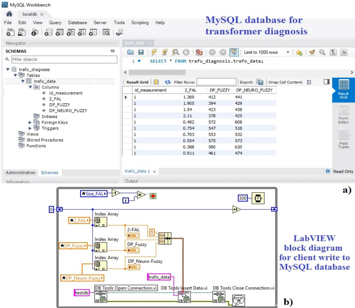
Figure 13: MySQL database connection: a) Table of results in MySQL database, b) block diagram of the client write software module into database
