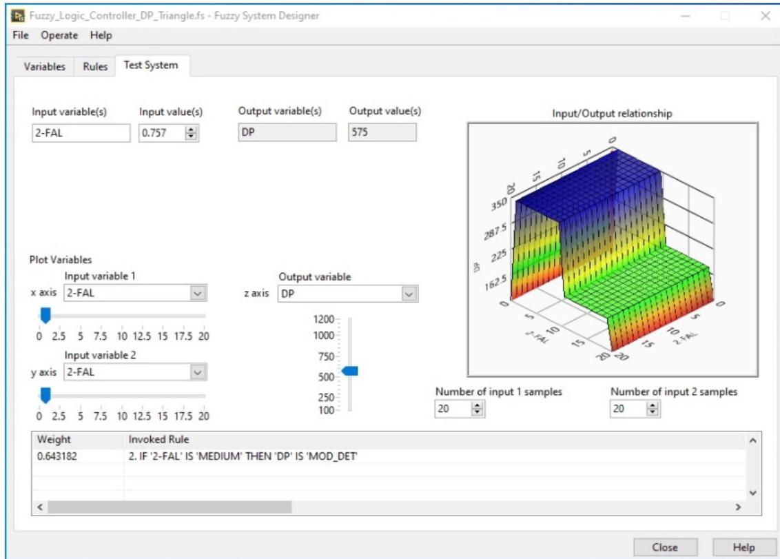
Figure 6: Surface viewer of DP result based on triangular fuzzy logic controller
