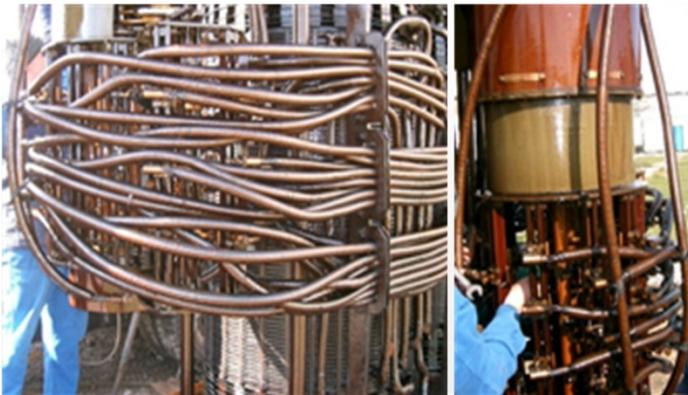
Figure 15: On-load tap-changer selector switch
