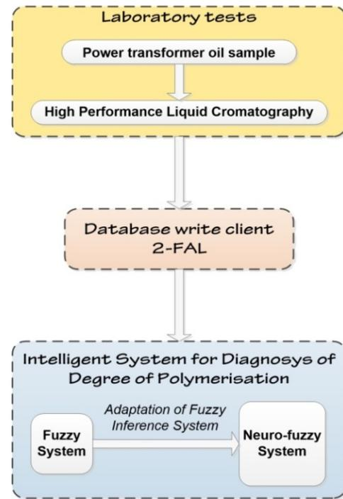
Figure 2: General scheme for the proposed system for diagnosis of DP
