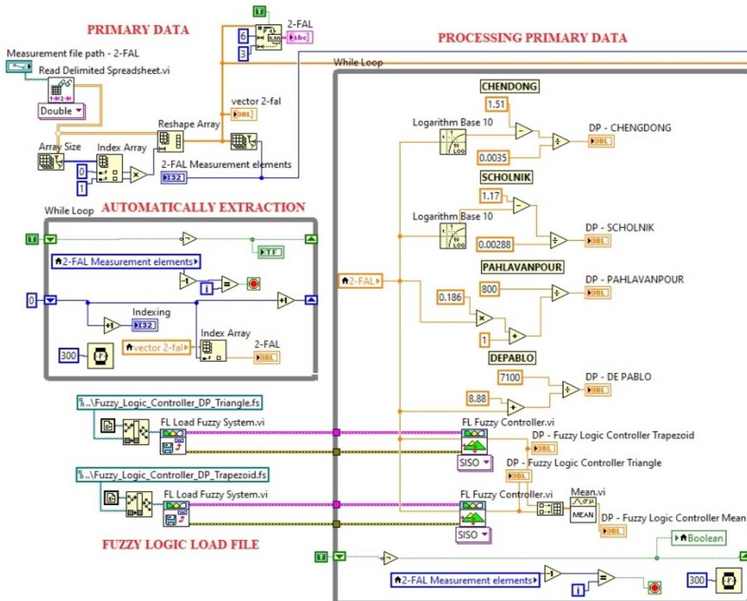
The software block diagram of the software application developed in LabVIEW for the main stages of the DP diagnostic software application is presented in Figure 8.
