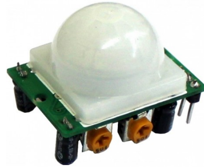
Figure 3: HC-SR501 PIR proximity sensor [9]
