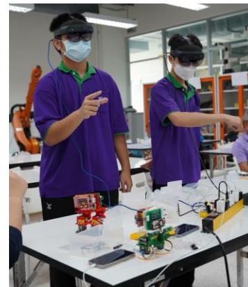
Figure 23: Users send robot commands to the real robot via HoloLens 2
