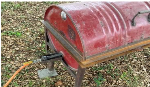
Figure 2: The gas inlet part of the kiln and the kiln not yet completely closed
