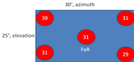
Fig.9. Number of Rx beams required in different locations of transmitting beam (Red areas) in the Field of Regard (Blue area: 30° azimuth x 25° elevation).
