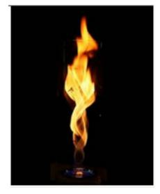
Figure 8. Evaluation of experimental prototype. There are three flame zones; laminar zone (lower), transition zone (middle), and turbulent zone (upper).
