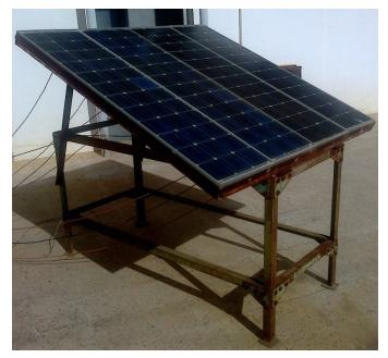
Figure 7. Photovoltaic system mounted at our laboratory.
