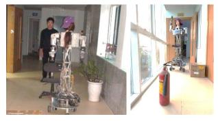
Figure 13: Approaching a human target and avoiding obstacles
