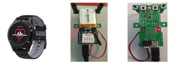
Figure 18: Smartwatch and ZigBee sensors
