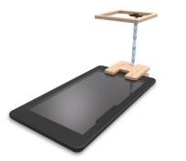
Figure 5. When the user can't hold the phone steadily with their hands, the supporting fixture make the response time from scanning faster
