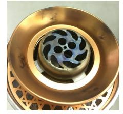
Figure 6. The metal cover on top of the torch: The central hole is the exit of the main flame. There is four side flame exit. The outer leaf-shaped opening is air inlet of the mixing zone.
