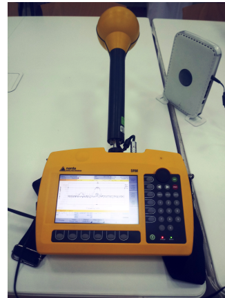
Figure 3: Measurements of radio frequency exposure from Wi-Fi access point
