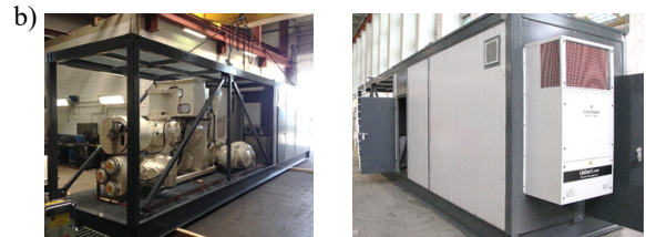
Figure 8. 3D CAD model of 110 kV grid impedance measurement system (a) and photos of the current construction status (b)
