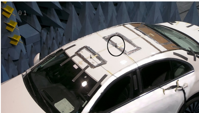
Figure 3: Photograph of the antenna-under-test, installed in VISTA. The AUT (indicated by the black circle) is connected to the Tx/Rx path of the UE, while the second Rx path is matched with a 50 Ω load.
