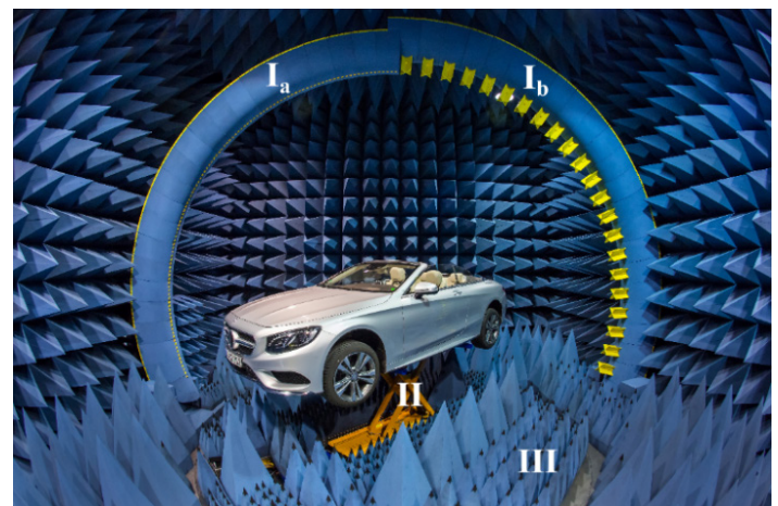
Figure 1: Photograph of VISTA with a car installed for automotive antenna measurement: Multi-probe antenna arch for the frequency range from 400 MHz up to 6 GHz (Ia) and from 70 MHz to 400 MHz (Ib). II: A customized vehicle lift elevates the car-under-test to the centre of the measurement arch 2.30 m above ground. III: The EMC-compatible turntable is used for azimuthal rotation with an accuracy of 0.1°.
