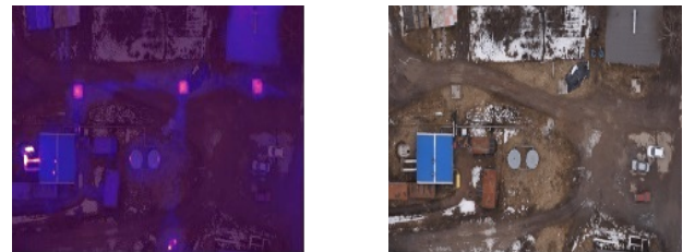
Figure 2. Detection of the places technological heat energy losses through un-insulated unions
