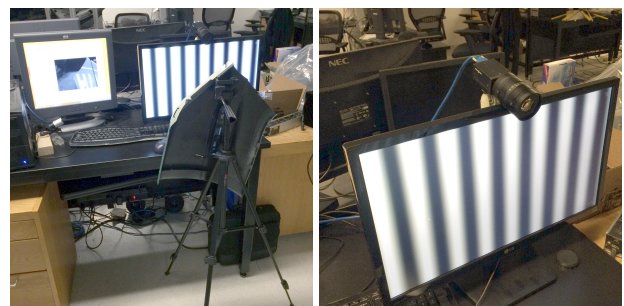
Figure 13: Camera with fringe pattern screen and test part on tripod
