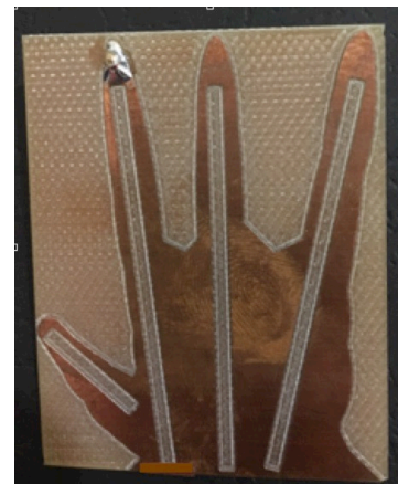
Figure 11: Antenna prototype with slots with the feed at the 2 nd fingertip.
