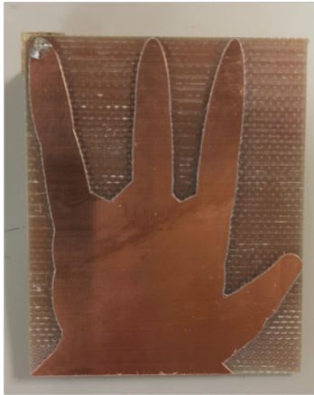
Figure 5: First feed scenario prototype at 4 th fingertip.
