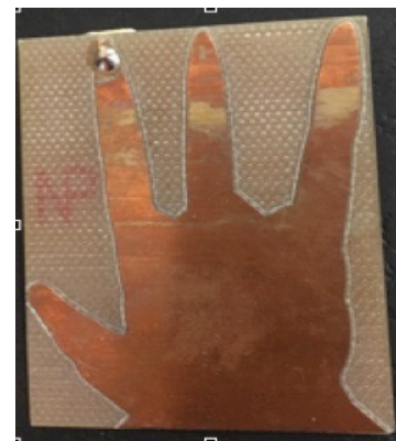
Figure 7: Antenna prototype with the feed at the 2 nd fingertip.
