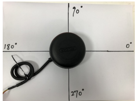
Figure 18: Use Rplidar to get the value of the angle
