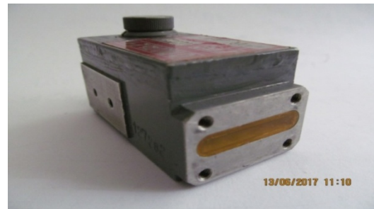
Figure 11: X-band VCO with the thermal compensation system of DR
