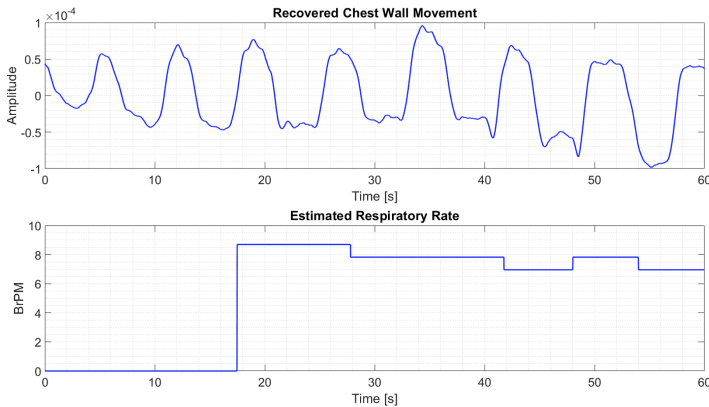
Figure 15: Experimental set-up. Life signals, breathing rate, of the fugitive detected behind the wall. Normal breathing conditions.
