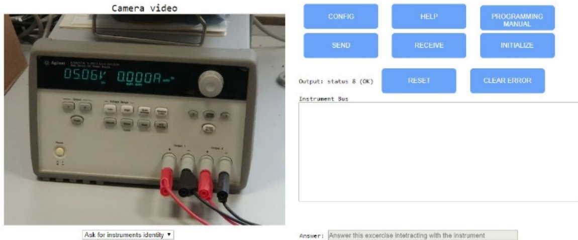
Figure 6: Main web interface GPIB SCPI experience
